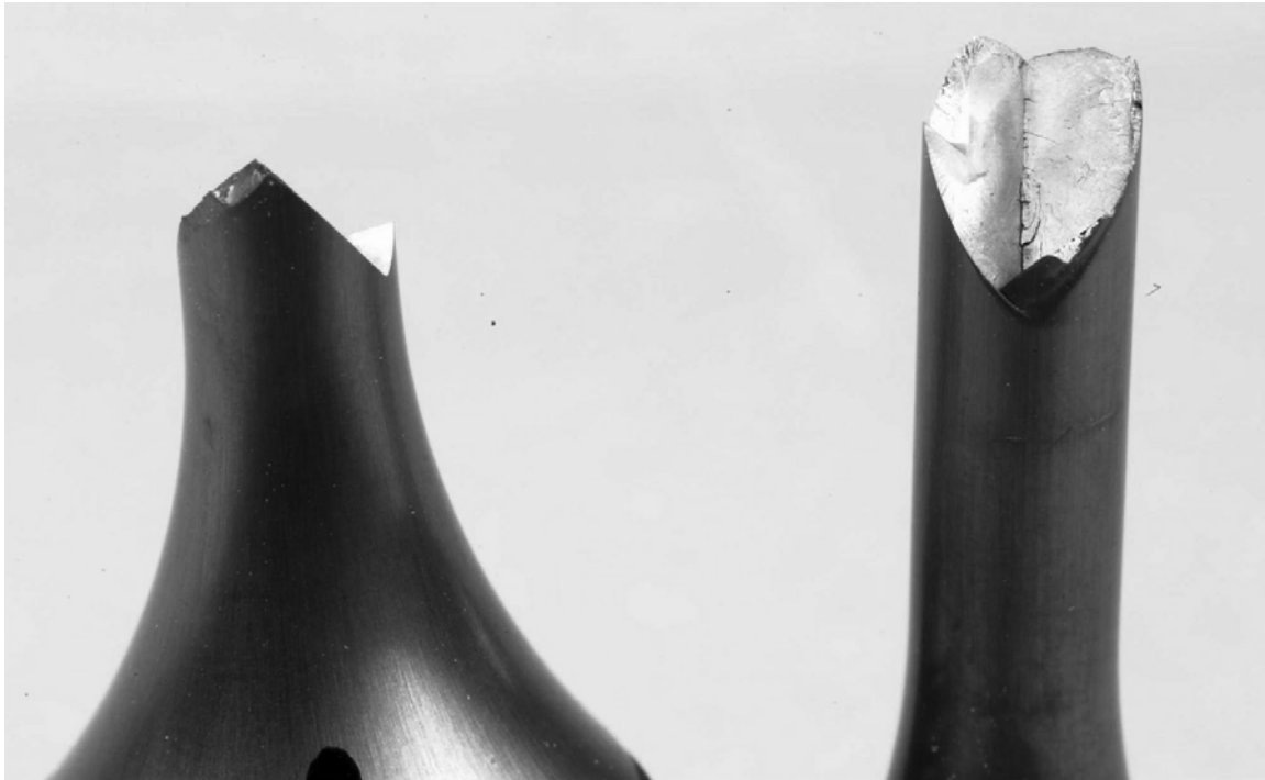
Figure 5: Fracture Surface of PWA 1484 (60 Hz).
